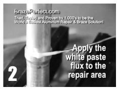
Apply paste flux to repair area. PRO TIP: Use the wire to apply flux and reduce contámination.
